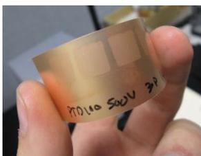
Fig. 5: Printed, flexible capacitor layers for energy storage applications
