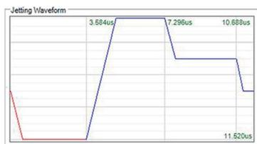
Fig. 3 Waveform used for printing dielectric monomer inks.
