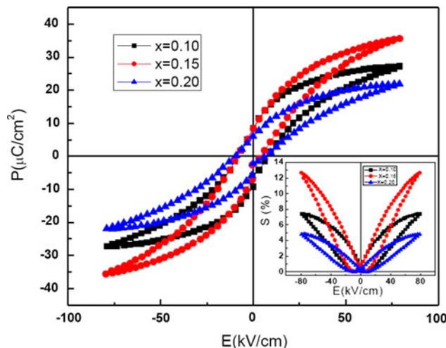
**Fig. 3** Room temperature  $P$ – $E$  and  $S$ – $E$  loops (inset) of  $[(\text{BaZr}_{0.2}\text{Ti}_{0.8})\text{O}_3]_{1-x}-[(\text{Ba}_{0.7}\text{Ca}_{0.3})\text{TiO}_3]_x$  ( $x = 0.10, 0.15, 0.20$ )—(BZT–BCT) ceramics sintered at  $1600^\circ\text{C}$
