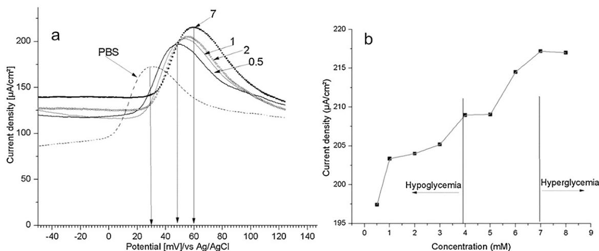
**Fig. 4.** Typical cyclic voltammograms of MAPLE-deposited CPPOPP thin films on SPE-110 at 300 mJ/cm<sup>2</sup> laser fluence in case of 0.5 mM, 1 mM, 3 mM, and 7 mM glucose concentrations in PBS: (a) Current density vs. potential for PBS and PBS and glucose vs. Ag-pseudoreference electrode (equivalent with Ag/AgCl), and (b) Peak current density vs. concentration in the range 0.5–8 mM glucose concentration.
