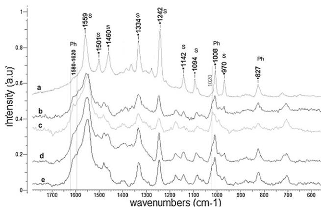
**Fig. 3.** Typical Raman spectra of CPPOPP dropcast (a) and MAPLE-deposited CPPOPP thin films at 200 mJ/cm<sup>2</sup> (b), 300 mJ/cm<sup>2</sup> (c), 400 mJ/cm<sup>2</sup> (d), and 500 mJ/cm<sup>2</sup> (e). S = Skeleton, Ph = Phenyl side groups (from Fig. 1).
