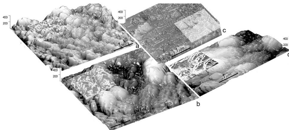
**Fig. 2.** Typical AFM micrographs of CPPOPP MAPLE-deposited thin films at  $200\text{ mJ/cm}^2$  (a),  $300\text{ mJ/cm}^2$  (b),  $400\text{ mJ/cm}^2$  (c), and  $500\text{ mJ/cm}^2$  (d). The height of AFM profiles is given in nanometers.
