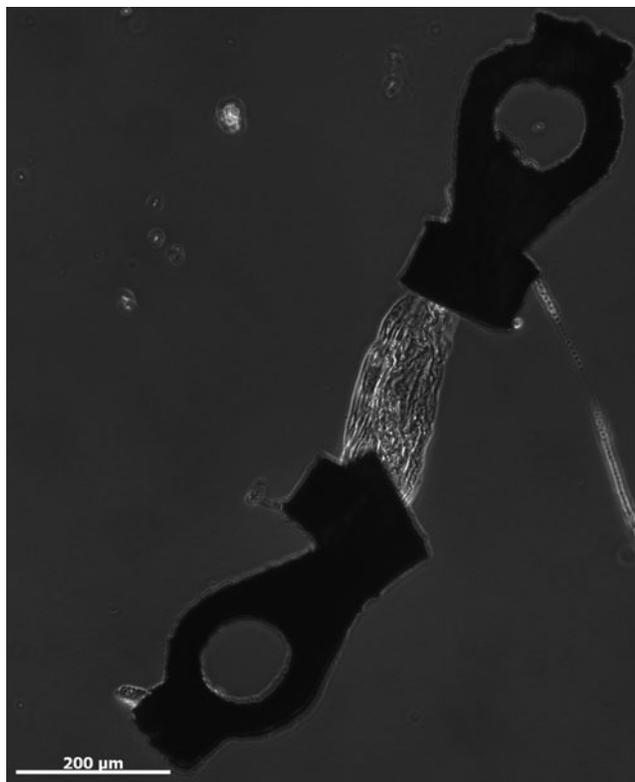
**FIG. 5.** A cellular fiber test section gripped with T-clips for mechanical evaluation on a custom microscope-based, single-fiber mechanics rig.
