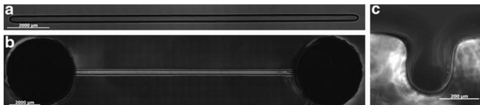
**FIG. 1.** (a) Top view of a growth channel laser micromachined into agarose gel, demonstrating consistent dimensions along its 1.65-cm length. (b) Two 4-mm-diameter collagen sponge disks are inserted into each end of the growth channel to act as anchor points for the developing cellular fiber. (c) A cross section of growth channel demonstrates its depth and three-dimensional structure.
