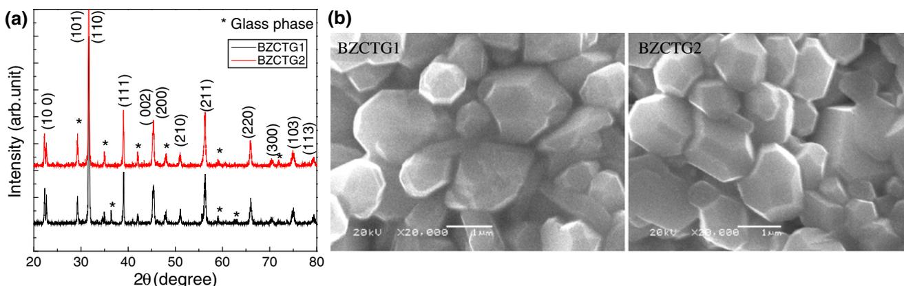
**Fig. 1** Room temperature XRD patterns of glass–ceramics [ $0.10 \text{ BaO} + 0.4 \text{ B}_2\text{O}_3 + 0.5 \text{ ZnO}$ ], [ $0.3 \text{ BaO} + 0.6 \text{ B}_2\text{O}_3 + 0.1 \text{ ZnO}$ ]— $[(\text{BaZr}_{0.2}\text{Ti}_{0.80})\text{O}_3]_{1-x} - [(\text{Ba}_{0.70}\text{Ca}_{0.30})\text{TiO}_3]_x$ —BZCTG1, BZCTG2, sintered at  $900^\circ\text{C}$ , with  $2\theta$  angle ranging from  $10$  to  $80^\circ$
