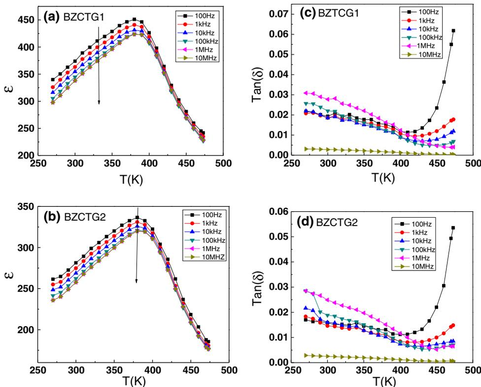
**Fig. 3** a, b The temperature dependence of the dielectric permittivity of glass–ceramics [0.10 BaO + 0.4 B<sub>2</sub>O<sub>3</sub> + 0.5 ZnO], [0.3 BaO + 0.6 B<sub>2</sub>O<sub>3</sub> + 0.1 ZnO] – [(BaZr<sub>0.2</sub>Ti<sub>0.80</sub>)O<sub>3</sub>]<sub>1-x</sub> – [(Ba<sub>0.70</sub>Ca<sub>0.30</sub>)TiO<sub>3</sub>]<sub>x</sub>—BZCTG1, BZCTG2, sintered at 900 °C at 100–1 MHz. c, d The
