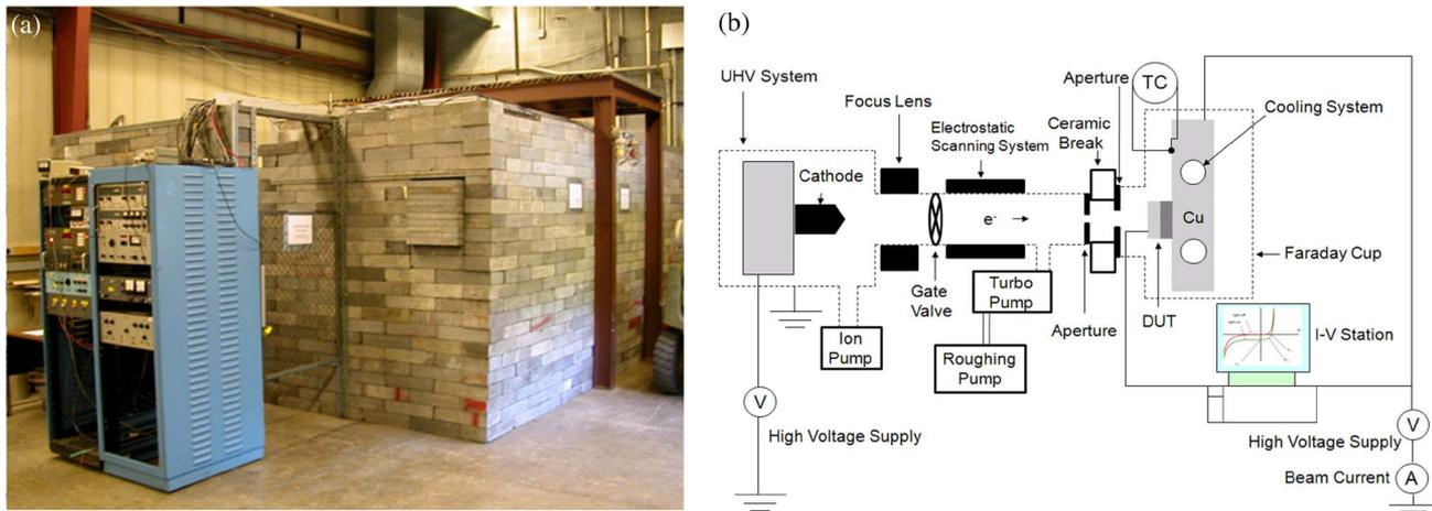
Fig. 1. Customized LEEA at Rensselaer Polytechnic Institute: (a) outlook picture and (b) schematic of LEEA. Here, TC is for thermocouple, DUT is for device under test, and UHV is for ultrahigh vacuum.
