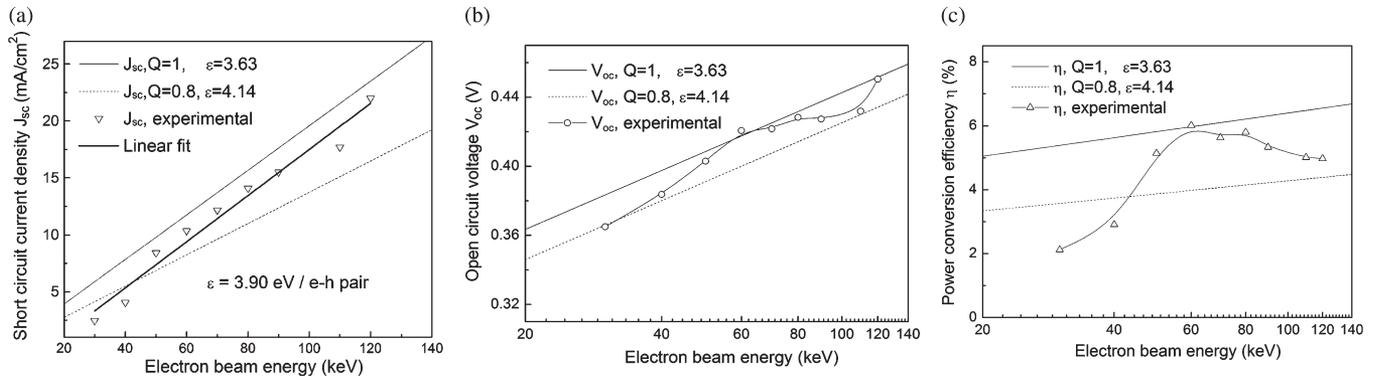
Fig. 4. Experimental and calculated betavoltaic performance as a function of electron beam energy (a)  $J_{sc}$  versus  $E$ , (b)  $V_{oc}$  versus  $E$ , and (c)  $\eta$  versus  $E$ . The boundary limits are calculated by using  $r = 0.1$  and  $n = 1.90$ . Here, the electron beam current density is  $0.79 \mu\text{A}/\text{cm}^2$  for experimental data.
