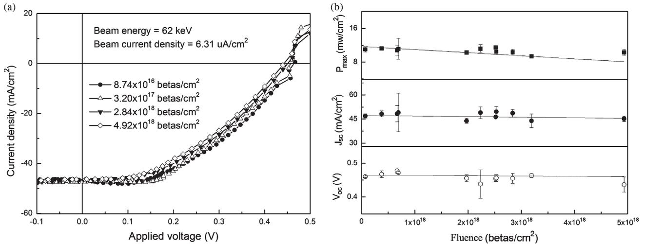
Fig. 6. Effect of radiation damage on the betavoltaic performance of Si space solar cells under the bombardment of electrons with the beam energy of 62 keV and the beam current density of 6.31  $\mu\text{A}/\text{cm}^2$ . (a)  $I$ - $V$  characteristics at different fluence levels. (b) Maximum output power  $P_{\text{max}}$ , short-circuit current density  $J_{\text{sc}}$ , and open-circuit voltage  $V_{\text{oc}}$  as a function of the fluence.
