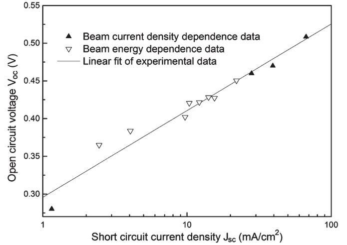
Fig. 3. Relationship of open-circuit voltage  $V_{\text{oc}}$  versus short-circuit current density  $J_{\text{sc}}$  for beam current density dependence and beam energy dependence.
