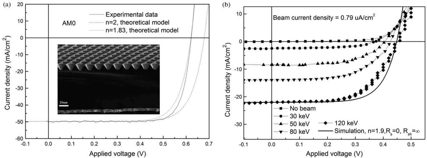
Fig. 2. (a) Photovoltaic and (b) betavoltaic characteristics of high-efficiency Si space solar cells. The inset in (a) is the tilt SEM cross-sectional image of as-received Si space solar cells and shows that the surface of the Si space solar cells was textured with inverted pyramid morphology.
