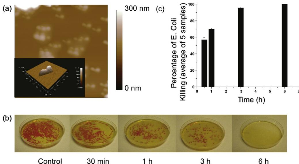
**Fig. 3.** (a) Atomic force microscopy of the bacterial colonies. Inset: 3D image of a single *E. coli*. (b) Agar plates marked with colonies of bacteria. The number of colonies after different incubation time of bacteria with AgCl is reported relative to control plates. (c) Percentage of *E. coli* killing upon incubation with AgCl for different amount of time.
