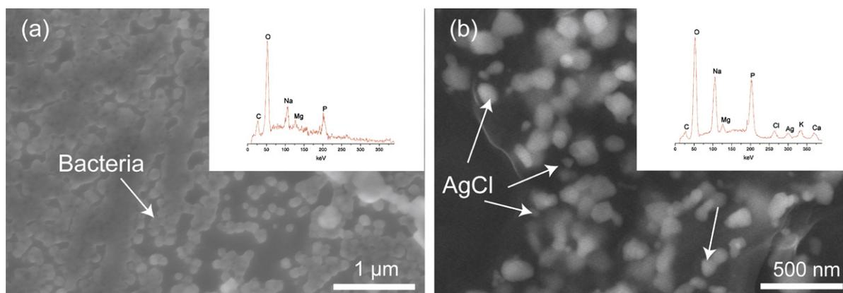
**Fig. 4.** (a) *E. coli* in SEM (arrows point to selected bacteria). Inset: the EDX spectrum of *E. coli*. (b) AgCl nanocubes embedded into a mass of cellular debris (arrows point to selected nanocubes). Inset: the EDX spectrum of the AgCl embedded in the cellular debris.
