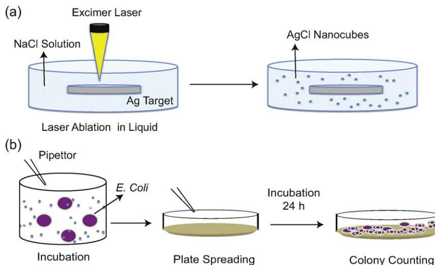
**Scheme 1.** Concept figure of the AgCl preparation by pulsed laser ablation of Ag target in NaCl solution (a) and their antibacterial testing using standard plating assay and gram negative bacteria (b).
